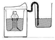
**Note:** You will only be able to siphon back into the machine until the water level is equal to that in the tub.
